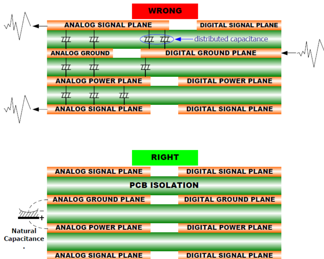
Fig.6 Cross section of PCB, the recommended separation for analog and digital plane.
